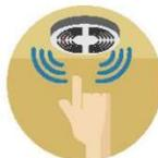
Test smoke alarms at least once a month by pushing the test button.
